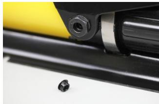
Remove the cap to expose the Allen set screw inside
