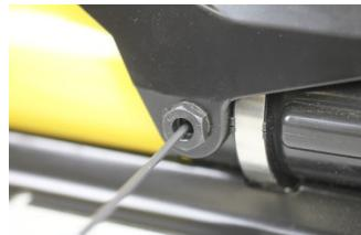
Insert a 1/8" Allen wrench to adjust the set screw. Clockwise will increase pressure / Counter-Clockwise to reduce pressure.
